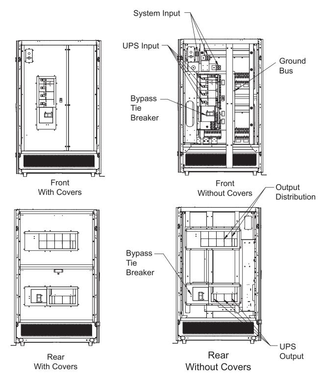
Figure 45 Liebert<sup>®</sup> NX<sup>™</sup> 480V paralleling cabinet main components—input, bypass and distribution circuit breaker configuration
